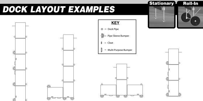
PlayStar Standard Docks are made from 4' x 6' modular sections which can be easily configured to meet any requirement.
