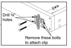
Remove the two carriage bolts from the frame as shown. Attach clip reusing the same hardware (note the orientation of the clips).
