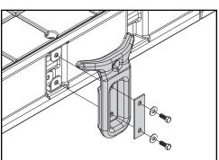
Attach Accessory Brackets to dock in desired location for Cleat. Use %" x 1" **STAINLESS STEEL** hex bolt to attach Cleat to the bracket. Do not over-tighten.
