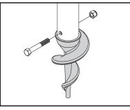
Drill one <sup>3</sup>/<sub>8</sub>" hole in pipe <sup>11</sup>/<sub>16</sub>" up from the end. Insert Auger into the pipe, align holes and finish drilling opposite side. Secure with the nut and bolt provided.
