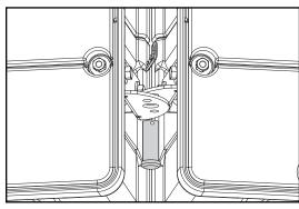
Connect sections with pin and clip
