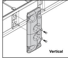
Attach Accessory Brackets to dock in desired location for Bumper. Use 3/8" x 1" **STAINLESS STEEL** hex bolt to attach Bumper to the bracket. Do not over-tighten.
