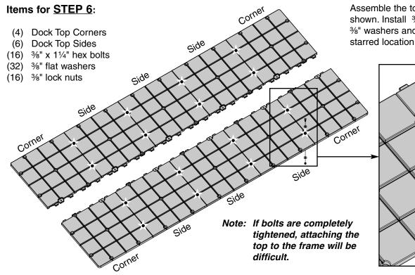
Assemble the tops into two halves as shown. Install 3/8" x 11/4" hex bolts, 3/8" washers and 3/8" lock nuts at each starred location. <u>Finger tighten only.</u>
