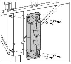
**To attach bumper to adjustable Dock Leg:** Use %" x 1" <u>GALVANIZED</u> hex bolt, %" washers, %" lock nuts from adjustable Dock Leg hardware to secure Bumper to Dock Leg as shown. Thank You for choosing PlayStar. Because it is our intention to make this a positive family experience, we have taken great care in preparing this product. Should you have any questions, or if we can assist you in any way, please call our friendly Customer Service Department for immediate action.
