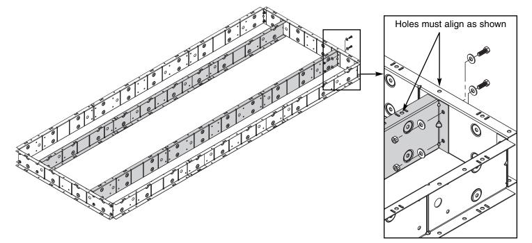
Install a Step 1 Rail Assembly as shown. Secure with
